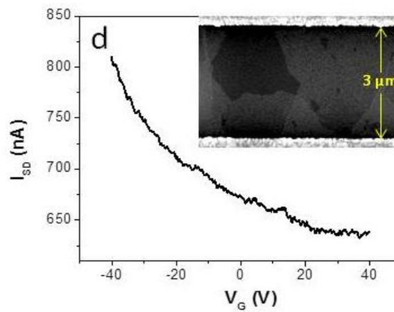
(c) The FET I-V curve of the crumpled GO FET device. Inset shows an SEM image of a crumpled GO across the electrode gap.
