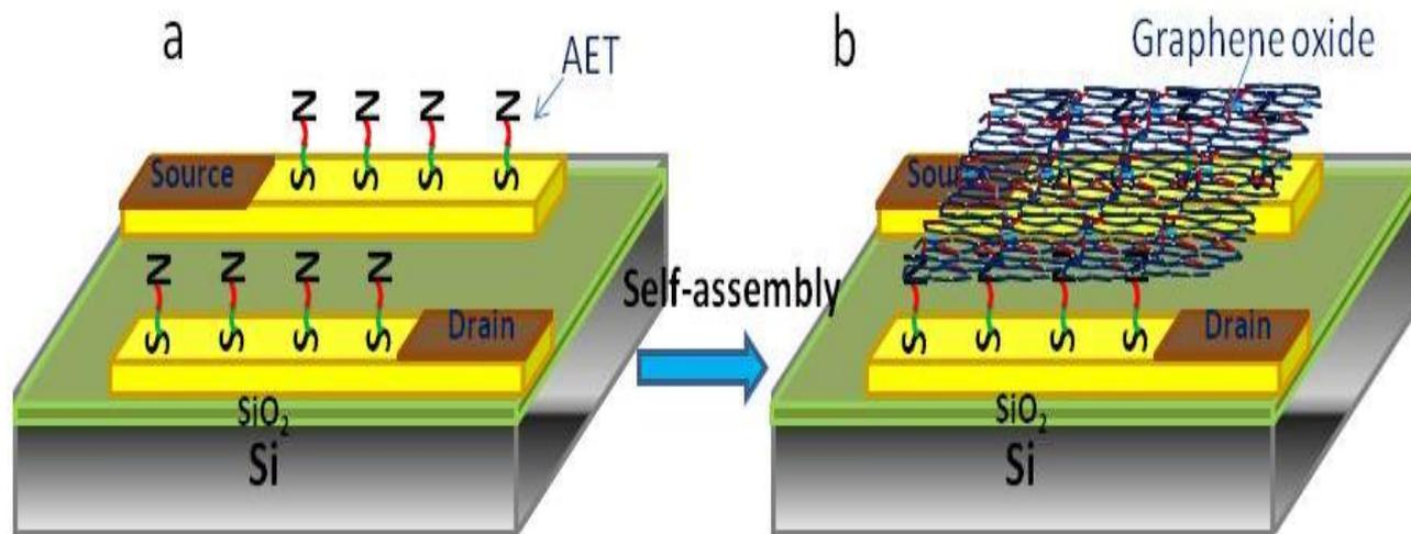
Schematic illustration of (a) a layer of AET coating on the electrode surface, and (b) self-assembly of GO sheets on the AET-modified electrodes.
